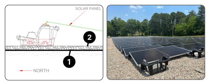
Suggested Ground Preparation for Proper Installation of Sollega FR510 Racking Units
